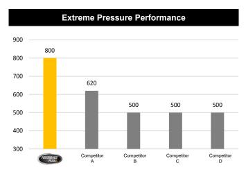
Performance Plus® delivers industry leading performance under extreme pressure loads in the 4-Ball Weld test. This exceptional performance protect critical components from damage under extreme conditions and therefore extend machine life and reduce maintenance costs.
